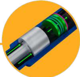
TOP VALVE (Open Valve)
